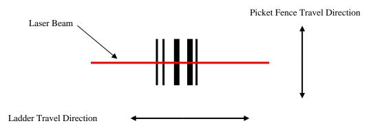
The SV unit must be programmed for the direction of travel of the codes being analyzed. If the codes are being scanned in a static condition, use picket fence travel direction.
