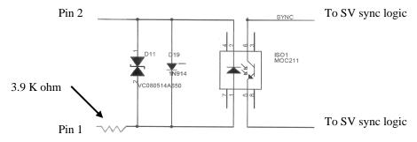
Figure C2 – Isolated Sync Input Diagram
