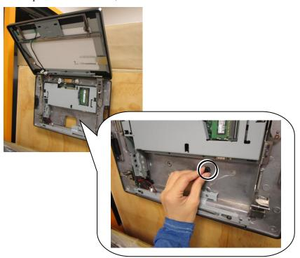
5. Connect the power cable, and other cables that you need. Make the cable pass through the cable exit on the bottom side of the ZT POS terminal.
