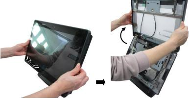
8. Pass the cable which you need into the cable exit.
