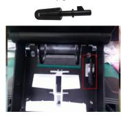
2. Insert the USB key into the keyhole, and then turn it clockwise.
