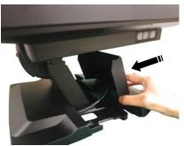
13. Make sure the cable could be pulled out of the cable exit from the bottom of the base.
