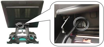
6. Push the latch with the thumb of the left hand, and then the touch monitor will release automatically.
