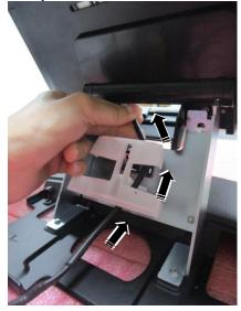
9. Connect the cables to the I/O port.
