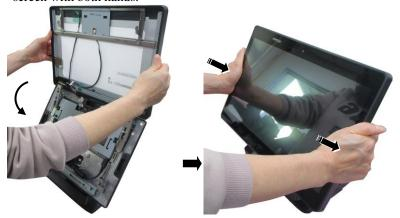
11. Rotate the screen to the horizontal position like below pictures.
