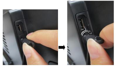
3. You can use the USB port after unlocking it. Be note that the USB key **CANNOT** be removed when the USB port is unlocked.
