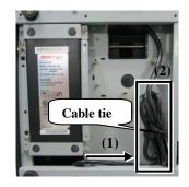
7. Place back the PoweredUSB compartment bracket into place, and then secure it using two fixing screws.
