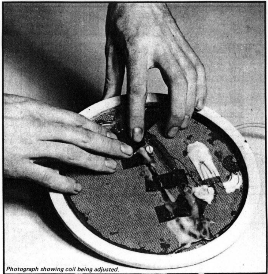
Fig.6 The construction of the search head - the key to the whole circuit.
